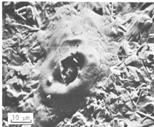
Figure 9 Mound formed during the high temperature oxidation of hot-pressed silicon nitride. The hole in the centre of the mound suggests that gas had issued forth from the mound. Microscopic examination indicates that a pit lies beneath the surface of the mound.
